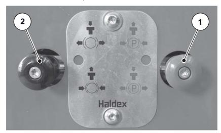
Figure 6.13: Releasing the parking brake
