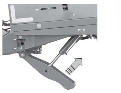
Figure 6.8: Retracting the support stand
