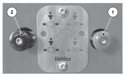
Figure 7.20: Releasing the manual parking brake
