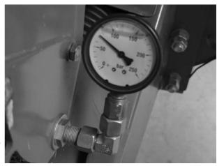
Figure 9.14: Pressure gauge at cable guide above towing bar
