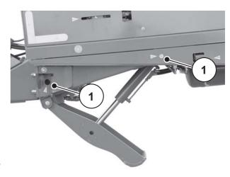
[1] Lubrication points: towing bar
