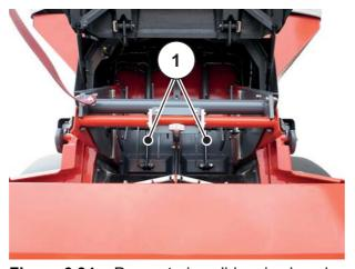
Figure 6.34: Pre-metering sliders in closed position
