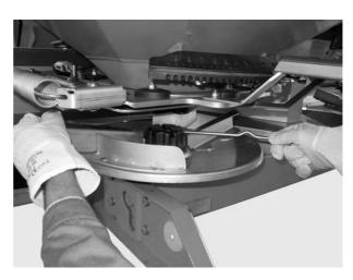
Figure 7.8: Undoing the cap nut
