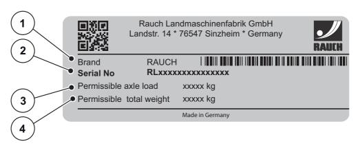
Figure 3.7: 2. Nameplate for towed machines
