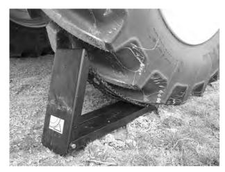
Fig. 55: Positioning the wheel chock
