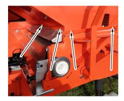
Now release the nuts of the metering shaft bracket [1] and fold down the brackets.
