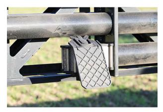
Fig. 46: Baffle in normal fertilizing mode
