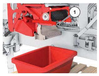
Fig. 52: Placing the spreader tank underneath
