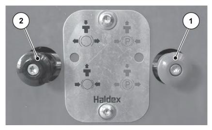
Fig. 43: Disengaging the parking brake
