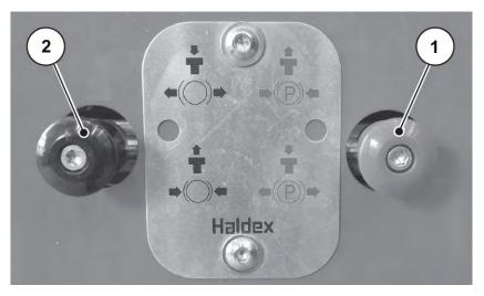
Fig. 53: Engaging the manual parking brake
