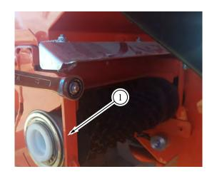
Since the metering rollers are often seated very tightly in the bracket, it is possible to insert a mounting lever or a shaft into the metering roller and use it to pry it out for easier removal.
