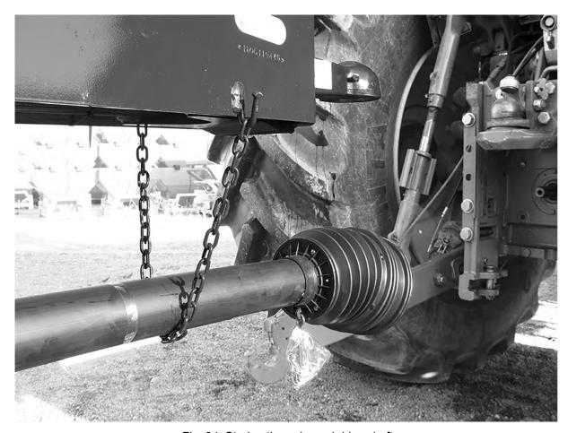
Fig. 24: Storing the universal drive shaft
