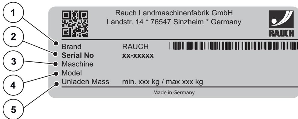
**Figure 3.6:** First nameplate for towed machines
