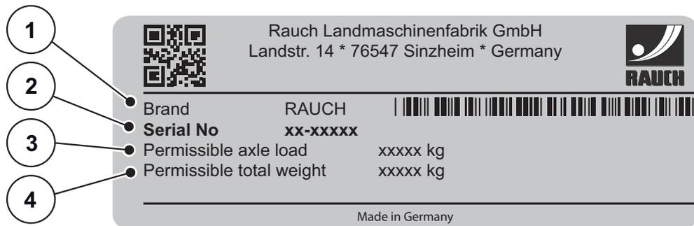
**Figure 3.7:** Second nameplate for towed machines
