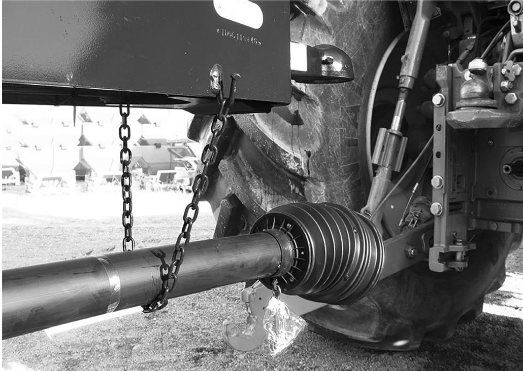
**Figure 6.6:** Storing the universal drive shaft
