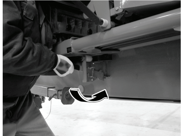
Fig. 30: Swing back the lever for the air duct rack
