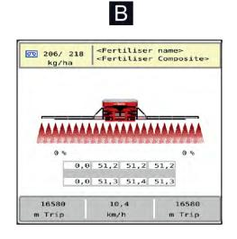
B Machine in spreading operation (START)
