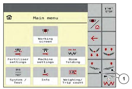
Fig. 15: Function keys for adjusting the boom inclination
