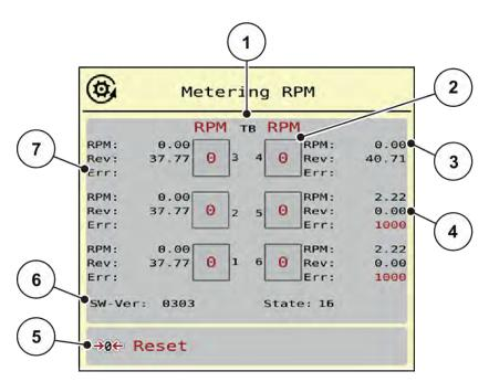
Fig. 19: Test/diagnosis; Example: Metering RPM
