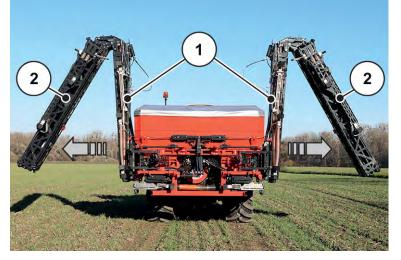
Fig. 14: Folding out the start sections and central sections
