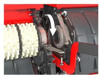
Fig. 38: Opening the metering roller bracket
