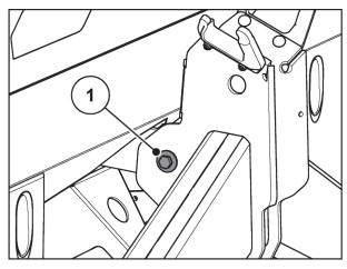
Fig. 55: Fastening the tie rod at the weigh frame
