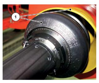
Fig. 4: Universal drive shaft guard
