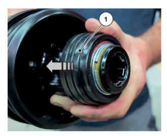
Fig. 21: Pulling back the pulling sleeve
