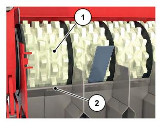
Fig. 60: Checking the distance between the cam wheels and the spreader tank
