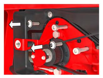
Fig. 37: Releasing screws on the motor
