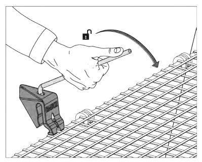
Fig. 57: Opening the protective grid lock
