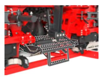
Fig. 26: Step retracted
