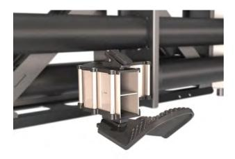
Fig. 47: Baffle in late fertilizing mode
