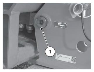
Fig. 64: Lubrication point of weighing spreaders
