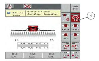
Fig. 20: DistanceControl button enabled
