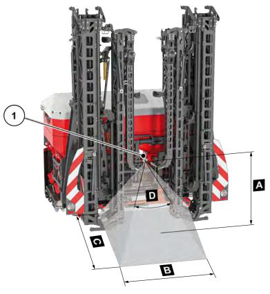
Fig. 14: Rear view camera field of vision when in transport position
