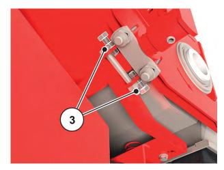
Fig. 61: Setting the distance between the cam wheels and the spreader tank
