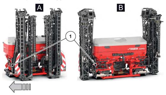
Fig. 40: Swiveling the swivel frame into the operating position
