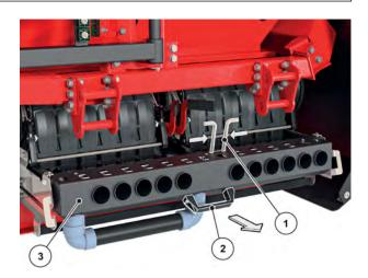
Fig. 49: Unlocking the injector cartridge
