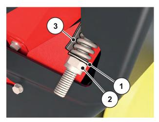
Fig. 62: Blower belt tensioning mechanism
