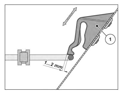
Fig. 58: Test dimensions for functional check of the protective grid interlock
