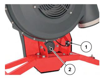
Fig. 65: Blower lubrication point
