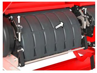
Fig. 35: Removing the metering roller cover
