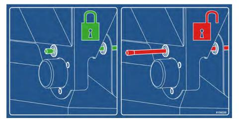
Fig. 39: Locking mechanism display
