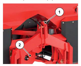
Fig. 52: Storage of the cables and hydraulic hoses
