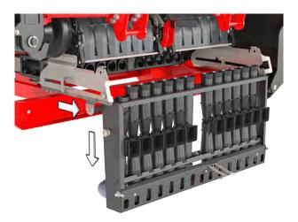
Fig. 50: Lowering the injector cartridge
