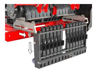
Fig. 31: Lowering the injector cartridge
