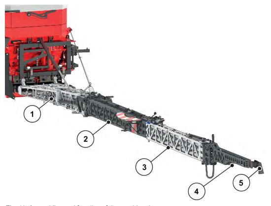
Fig. 11: Assemblies and function of the machine, boom
