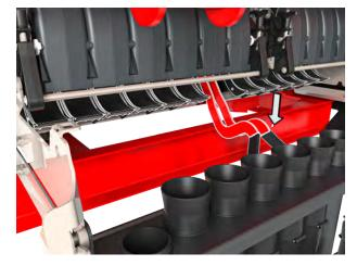
Fig. 34: Unlocking the metering tank
