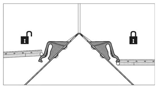
Fig. 56: Protective grid lock open/closed
