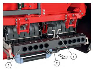
Fig. 30: Unlocking the injector cartridge
