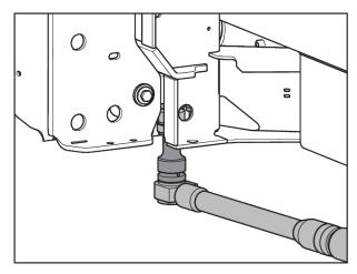
Fig. 54: Fastening the weigh cells (on the left side of the direction of travel)
