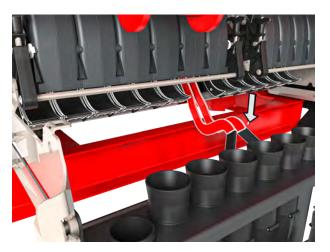
Fig. 51: Opening the locking mechanism of the metering tank
