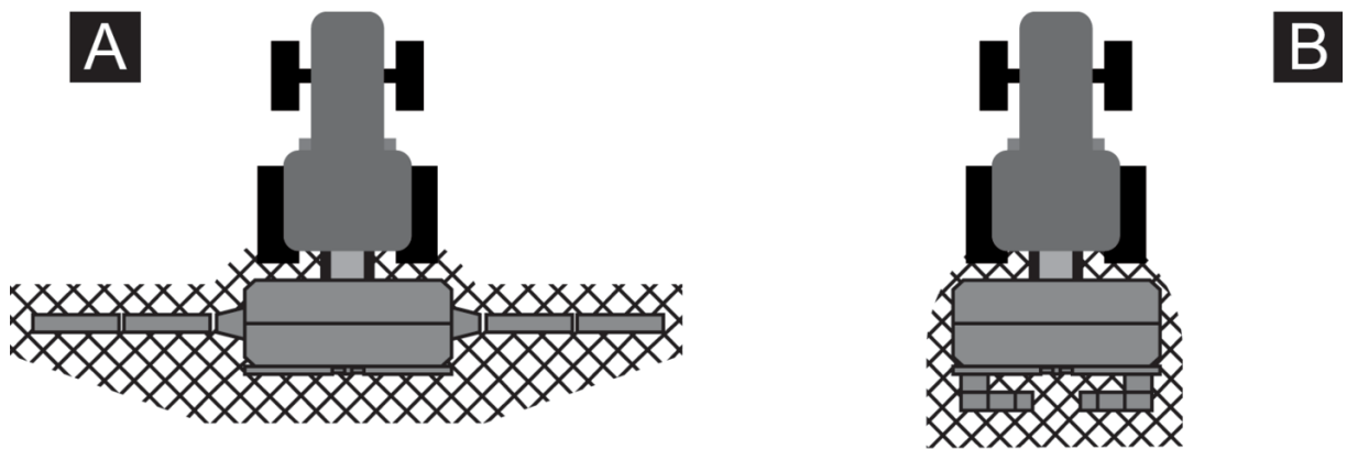
Fig. 1: Hazard zone when devices are attached
