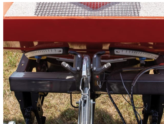
Fig.3: DfC scale in the field of vision
