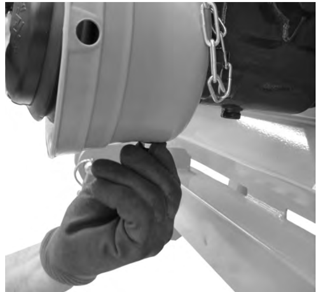
Fig. 9: Inserting a hexagon head screw
