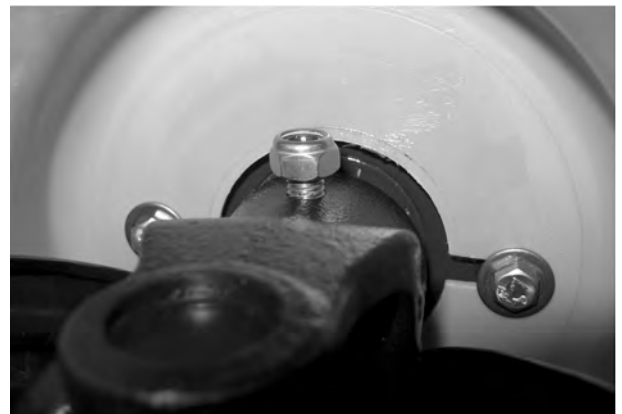
Fig. 10: Tightening the hexagon head screw
