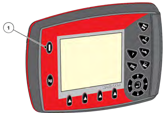
Fig. 16: Switching on the control unit
