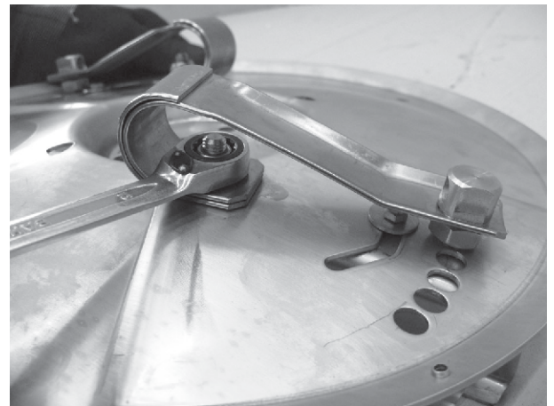
Fig. 94: Attachment of the flat spring
