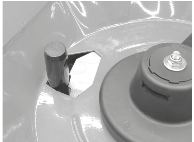
Fig. 68: Lower link pin in metering opening
