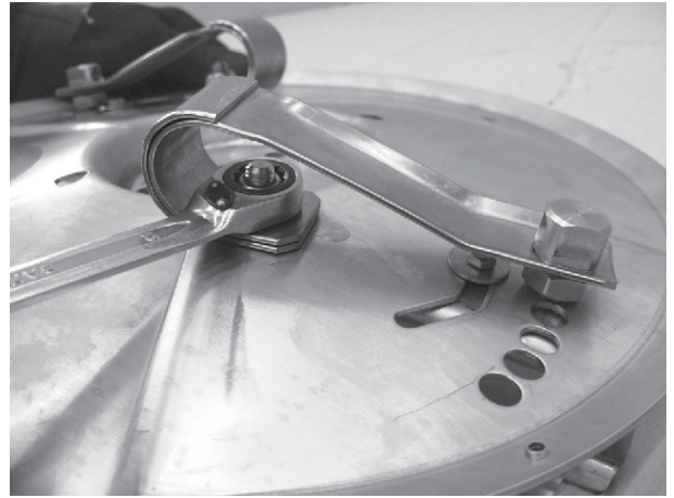
Fig. 86: Removing the screws
