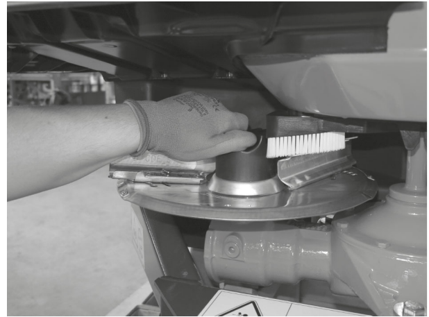
Fig. 38: Screw on the cap nut
