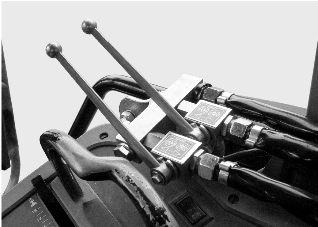
Fig. 28: Metering slide actuator of the two-way unit
