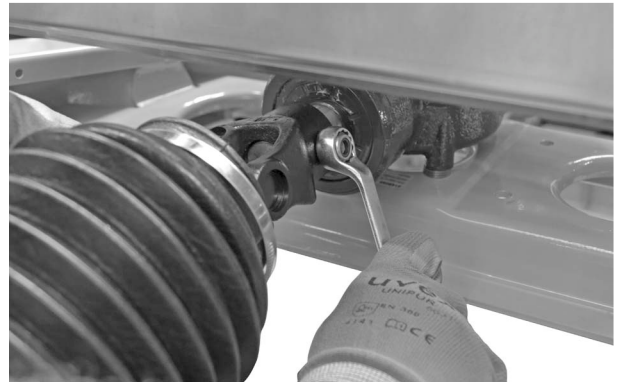
Fig. 13: Connecting the universal drive shaft
