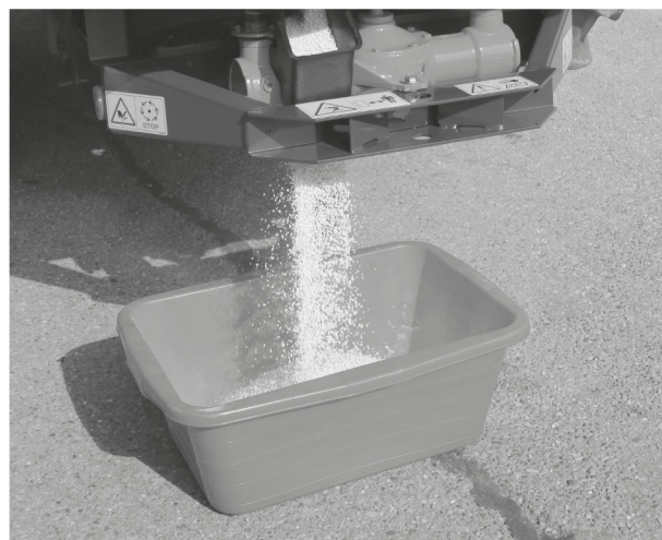
Fig. 37: Implementing the calibration test
