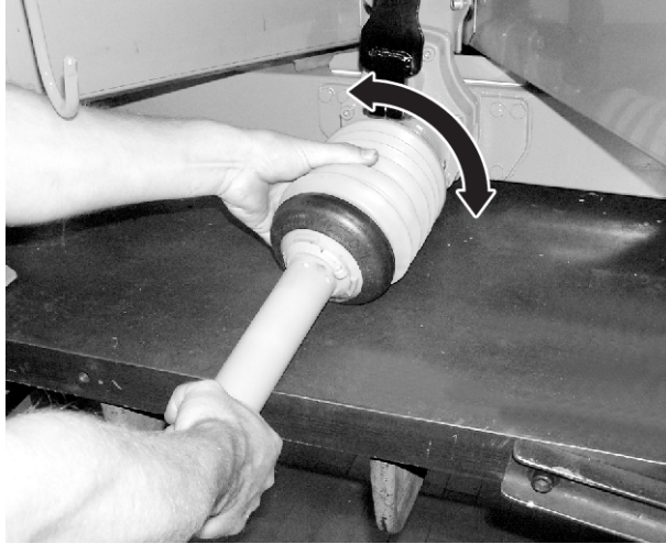
Fig. 20: Attaching the universal drive shaft guard
