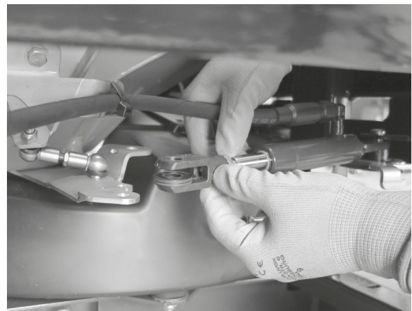
Fig. 71: Pull out the hydraulic cylinder
