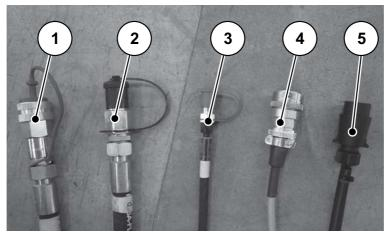
Figure 7.3: Mineral fertiliser spreader connection lines
