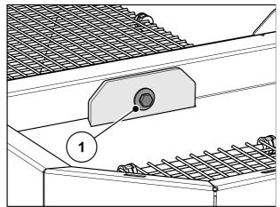
Tighten the screw connection with a torque wrench (Tightening torque = 65 Nm).
