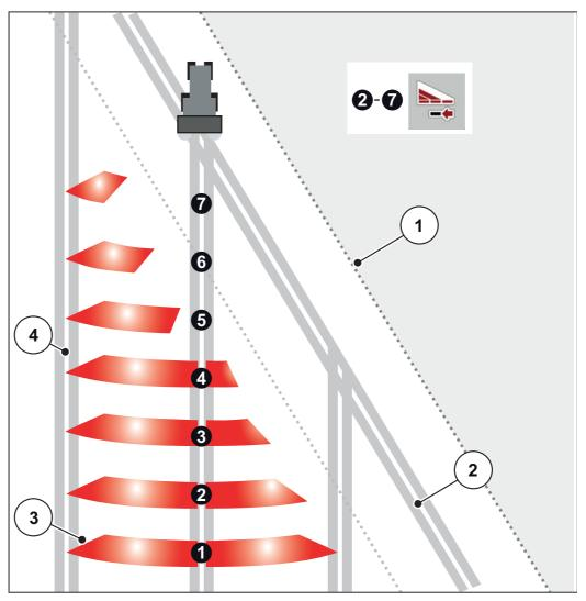
Figure 8.8: Automatic section control
