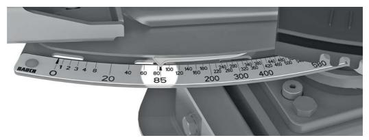
Figure 9.16: Metering slide pointer on position 85
