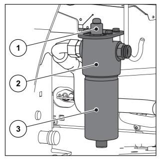
Figure 9.18: Hydraulic pressure filter
