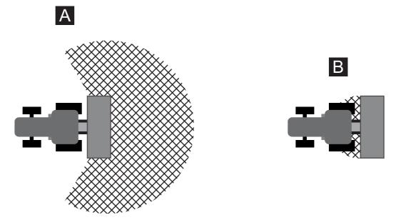
Figure 3.1: Hazard zones around attachment units
