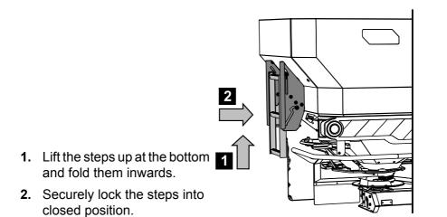
Figure 7.11: Folding in the steps in closed position
