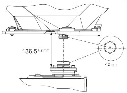
Figure 9.8: Checking the position of the spreading disc hub
