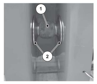
**Figure 7.1:** Position of the distance washers when installing the machine (AXIS H 50.2 EMC, category III)
