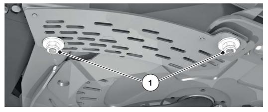
Figure 9.15: Scale mounting screws
