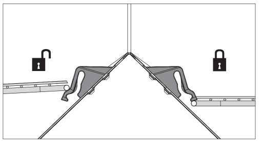
Figure 9.5: Protective grid lock open/closed
