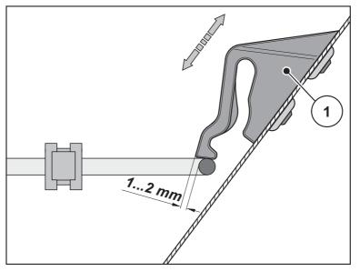
Figure 9.7: Test dimension for functional check of the protective grid lock
