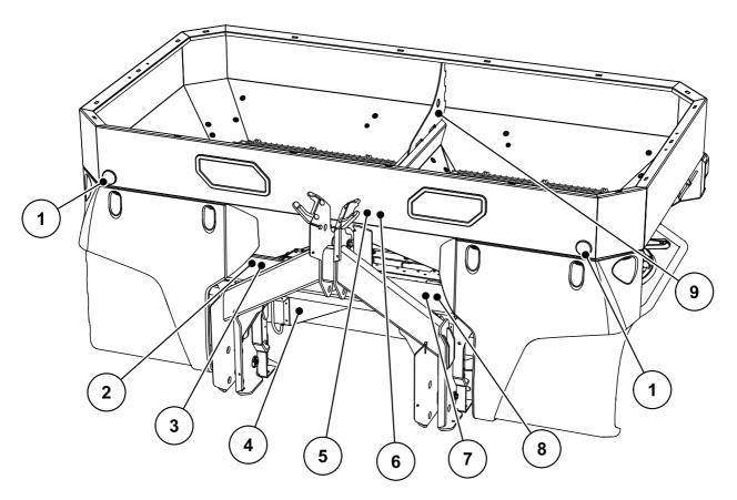
Figure 3.2: Safety equipment, warning and instruction stickers, front
