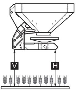
**Figure 7.6:** Maximum admissible mounting height V and H during normal and late fertilising
