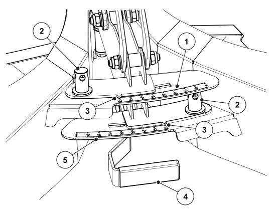
Figure 7.20: Setting the border spreading unit
