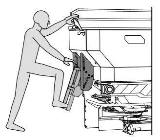
Figure 7.13: Climbing onto the machine with hopper cover
