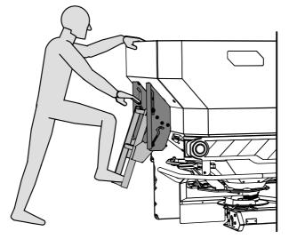
Figure 7.12: Climbing onto the machine without hopper cover
