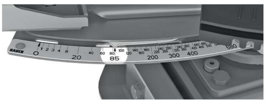
Figure 8.1: Scale for setting the spreading quantity
