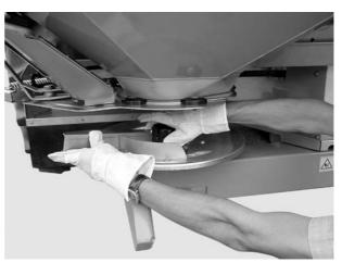
Figure 8.4: Unscrew the cap nut
