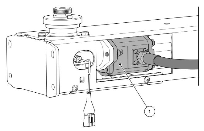
Figure 4.6: Hydraulic motor for spreading disc drive
