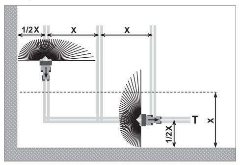
Figure 8.6: Limited border spreading
