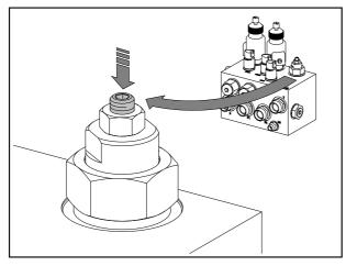
Figure 7.5: Set the adjustment screw at the hydraulic block for LS
