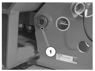
Figure 9.21: Weigh cells lubrication point
