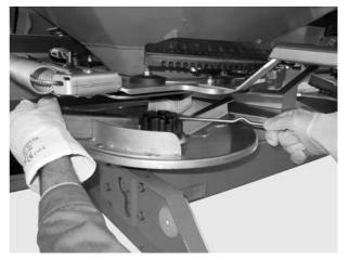
Figure 8.3: Loosen the cap nut
