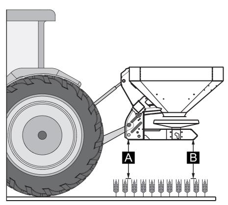
Figure 7.7: Mounting position and height during normal fertilisation
