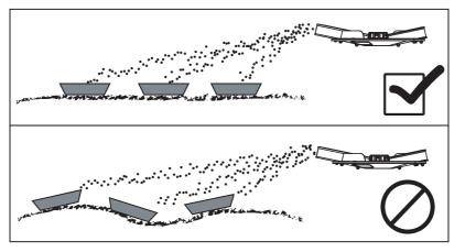
Figure 7.21: Layout of the collecting vessels
