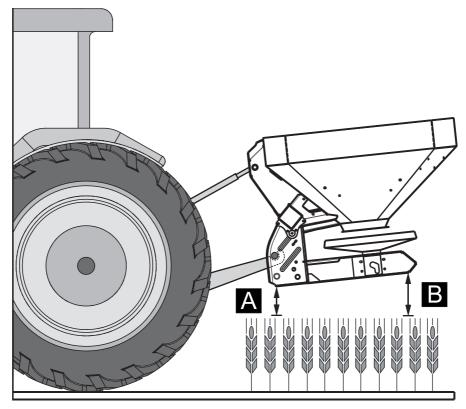
Figure 7.8: Mounting position and height during late fertilising
