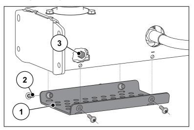
Figure 9.19: Gear oil filling and draining points
