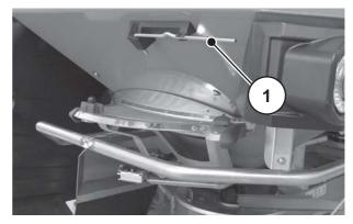
Figure 8.2: Adjustment lever
