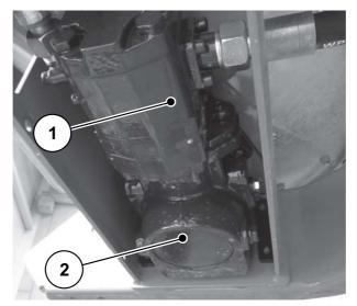
Figure 9.17: Hydraulic motor
