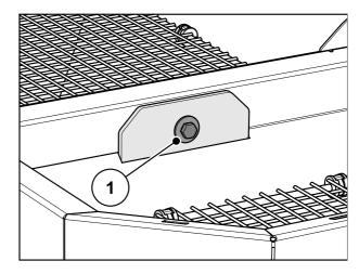
Tighten the screw connection with a torque wrench (Tightening torque = 65 Nm).
