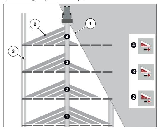
**Figure 8.21:** Spreading with section control (VariSpread)
