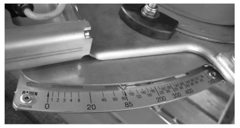
**Figure 2:** Scale for setting the spreading quantity
