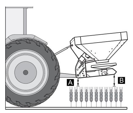
Figure 8.12: Machine mounted to the lower coupling point of the lower link
