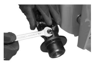
6. Remove lubricating nipples
