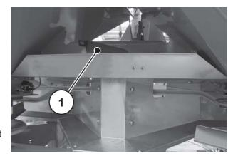
[1] Position of the calibration test chute
