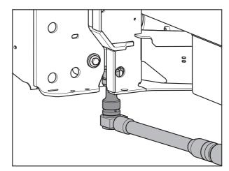
Tighten the screw connection with a torque wrench (Tightening torque = 300 Nm).
