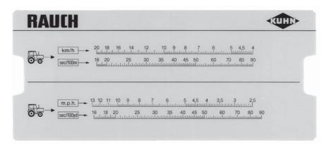
Figure 8: Scale for calculating the exact forward speed
