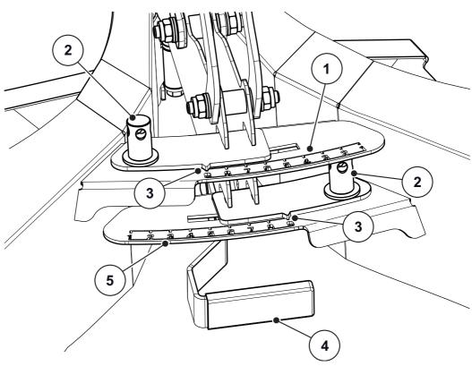
Figure 8.23: Setting the boundary spreading unit
