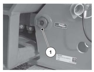
Figure 21: Lubrication point of weighing spreader
