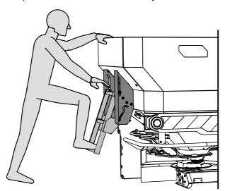
Figure 16: Climbing onto the machine without hopper cover
