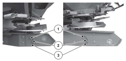
**Figure 9.10:** Gear oil filling and draining points; left:AXIS 20.2, AXIS 30.2, right AXIS 50.2
