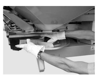
Figure 20: Screw on the cap nut
