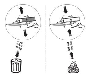
Figure 9.9: Use new self-locking nuts
