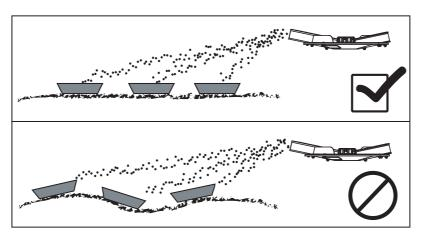
Figure 8.27: Layout of the collecting vessels
