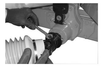
**11.** Retighten the lubricating nipples.
