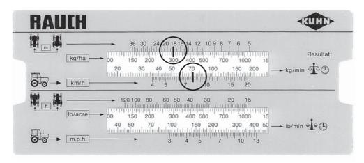
Figure 8: Scale for calculation of the nominal output quantity per minute
