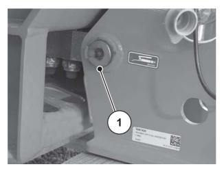
Figure 19: Lubrication point of weighing spreader
