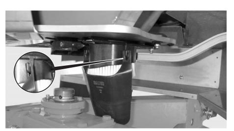
Figure 18: Attach the calibration test chute
