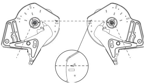
Figure 24: Checking the drop point
