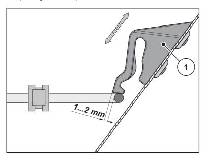
**Figure 9.3:** Test dimension for functional check of the protective grid lock
