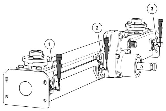
**Figure 4.5:** Mass flow control by measuring the torque of the spreading discs: AXIS-M 20.2/30.2/40.2 EMC
