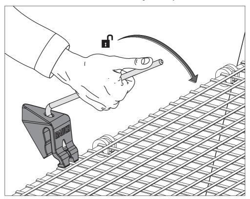
Figure 9.2: Open the protective grid lock
