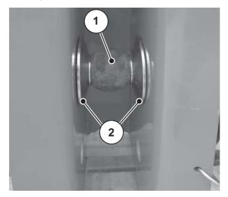
**Figure 8.7:** Position of the distance washers when installing the machine (AXIS 50.2, category III)
