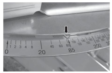
**Figure 26:** Metering slide pointer on position 85
