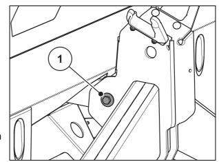
Tighten the screw connection [1] with a torque wrench (Tightening torque = 65 Nm).
