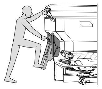
**Figure 18:** Climbing onto the machine with hopper cover
