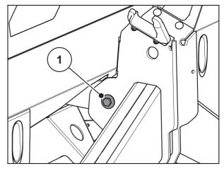
Tighten the screw connection [1] with a torque wrench (Tightening torque = 65 Nm).
