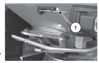
[1] Adjustment lever (hopper, left side according to direction of travel)
