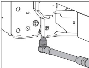
Figure 22: Fastening the weighing cell (on the left side of the direction of travel)
