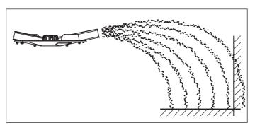
Figure 8.15: Full border spreading in normal fertilisation mode
