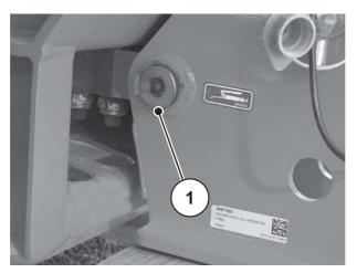
Figure 18: Lubrication point of weighing spreader
