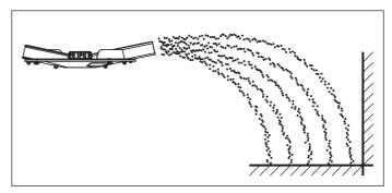
Figure 8.14: Limited border spreading in normal fertilisation mode
