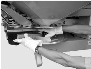
Figure 14: Screw on the cap nut
