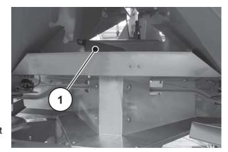
[1] Position of the calibration test chute
