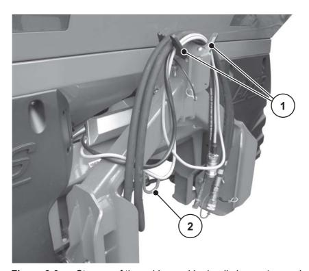
**Figure 8.6:** Storage of the cables and hydraulic hoses (example AXIS 50.2)
