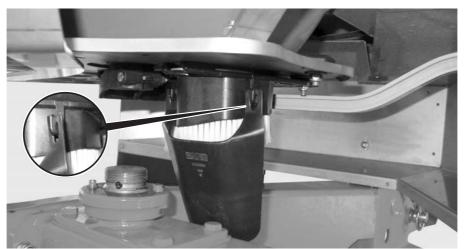
Figure 11: Attach the calibration test chute
