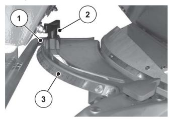
Figure 2: Scale for adjustment of the spreading quantity
