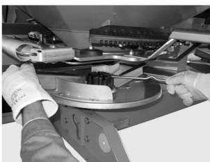
Figure 10: Loosen the cap nut
