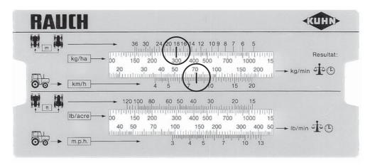
Figure 9: Scale for calculation of the nominal output quantity per minute
