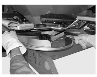
Figure 4: Loosen the cap nut
