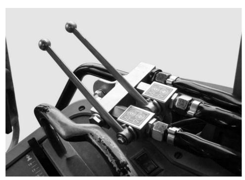
Slide actuator of the two-way unit
