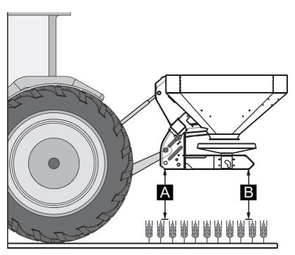
Figure 8.10: Mounting position and height during normal fertilisation
