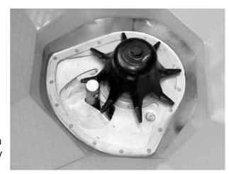
Insert a lower link pin with a diameter of 28 mm centrally into the metering opening.
