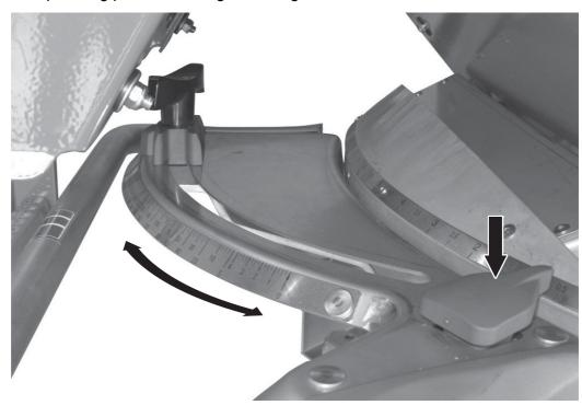
Figure 6: Adjustment centre for drop point
