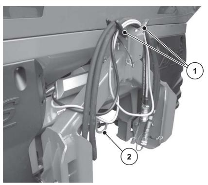
Figure 8.32: Storage of the cables and hydraulic hoses
