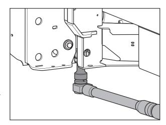
**Figure 19:** Fastening the weighing cell (on the left side of the direction of travel)
