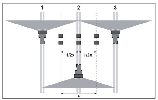
Figure 8.29: Layout for three passes
