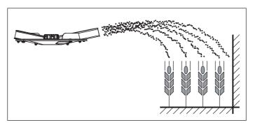
Figure 8.17: Limited border spreading during late fertilising
