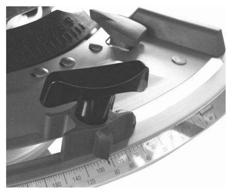
Figure 26: Adjustment scale of metering slide
