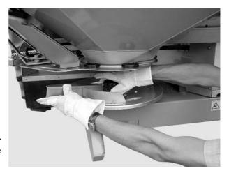
Figure 13: Screw on the cap nut
