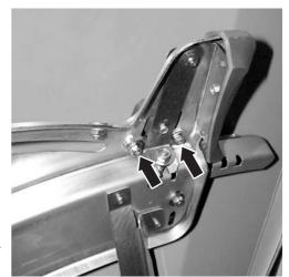
**6.** Release the adjustment plate underneath the "drop point pointer" (2 self-locking nuts).
