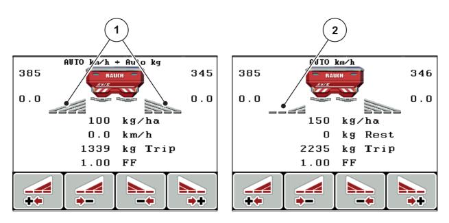
Figure 8.22: Display of the section status on the operating screen of the operating unit
