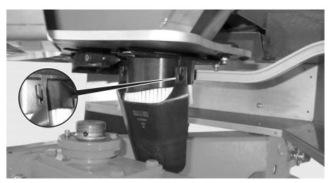
Figure 12: Attach the calibration test chute
