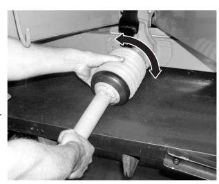
**Figure 6:** Put the universal drive shaft guard back on
