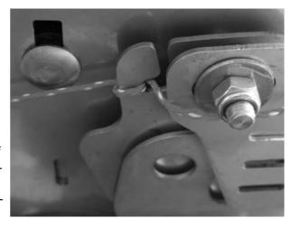
**Figure 30:** Attaching the string to the adjustment centre
