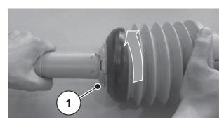
Figure 1: Loosen the universal drive shaft guard
