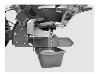
**6.** Position a collection vessel under the left output.
