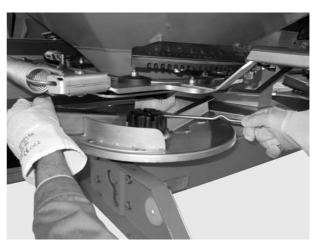
Figure 11: Loosen the cap nut
