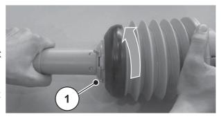
**Figure 8.1:** Loosen the universal drive shaft guard
