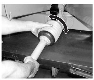
**Figure 8.4:** Put the universal drive shaft guard back on
