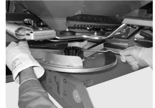
**1.** Remove the adjustment lever from the bracket.
