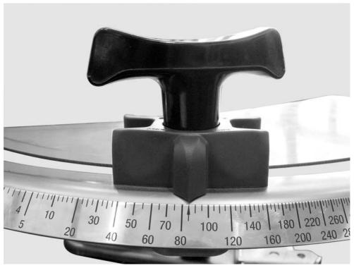
Figure 24: Adjustment scale of metering slide
