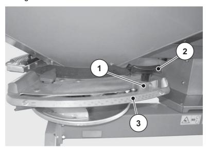
Figure 9: Scale for adjustment of the spreading quantity
