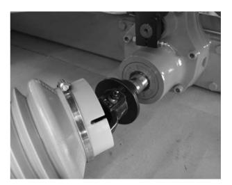
Figure 3: Push the universal drive shaft onto the transmission spigot
