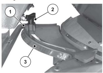
Figure 1: Scale for adjustment of the spreading quantity
