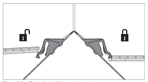
Figure 9.1: Protective grid lock open/closed
