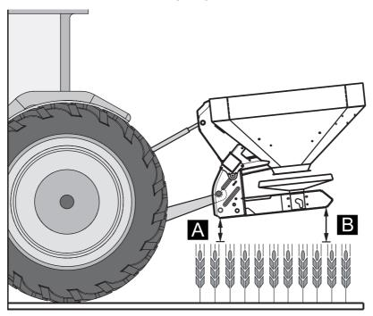
Figure 8.11: Mounting position and height during late fertilising
