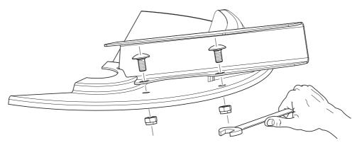
Figure 9.8: Loosen the screws on the spreader vane
