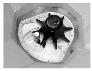
1. Insert a lower link pin with a diameter of 28 mm centrally into the metering opening.
