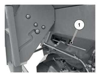
[1] Adjustment lever (hopper, left side according to direction of travel)
