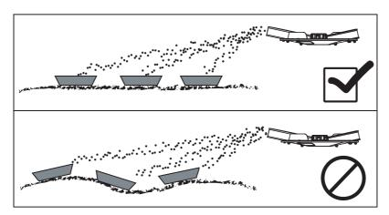
Figure 8.30: Layout of the collecting vessels
