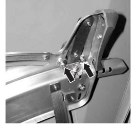
2. Release the adjustment plate underneath the "drop point pointer" button (2 self-locking nuts).
