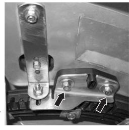
Figure 28: Loosen the drop point adjustment plate
