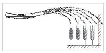
Figure 8.18: Full border spreading during late fertilising
