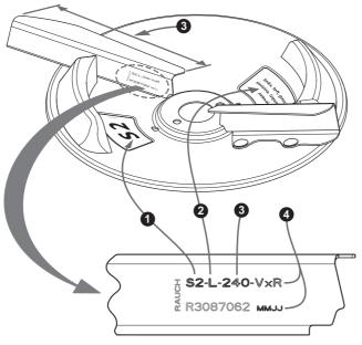
Figure 9.7: Spreading disc label
