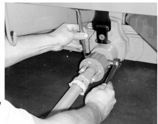
7. Tighten the hexagonal screw and nut using a size 17 wrench (max. 35Nm).
