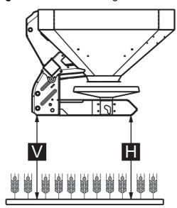
**Figure 8.9:** Maximum admissible mounting height V and H during normal and late fertilising
