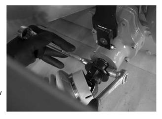
**10.** Tighten the hexagonal screw and nut using a size 17 wrench (max. 35Nm).
