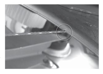
The triangular mark on the adjustment centre must coincide with the tensioned string.
