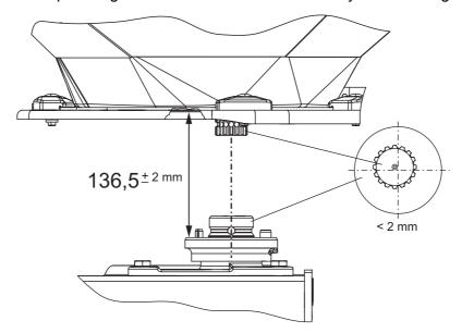
Figure 9.4: Checking the position of the spreading disc hub
