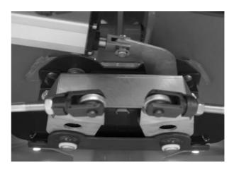
**18.** Hook the actuator back in position and secure.
