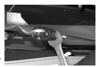
**4.** Hook the yoke in position and secure by tightening the locknut.
