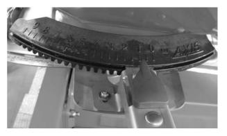
**Figure 9.30:** Checking the adjustment of the drop point
