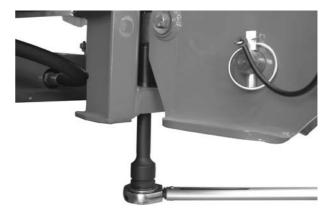
Tighten the bolted connection with a torque wrench (torque = 300 Nm).
