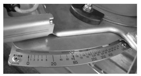
Figure 8.1: Scale for setting the spreading quantity
