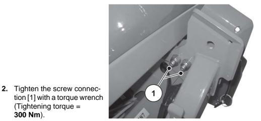
Figure 19: Fastening the tie rod
