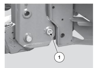
Figure 22: Lubrication point of weighing spreader
