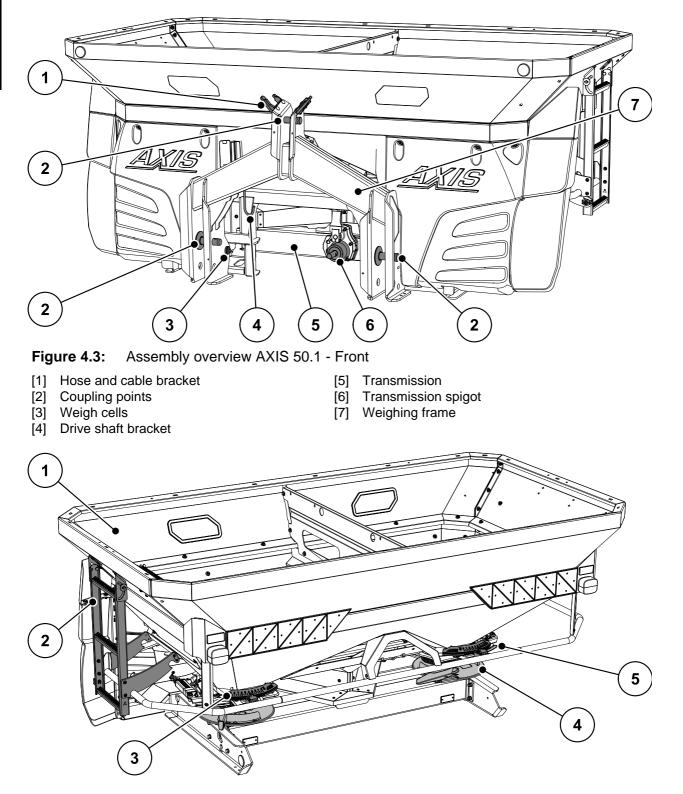
Figure 4.4: Assembly overview AXIS 50.1 - Rear
