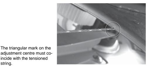
Figure 36: Markings on the adjustment centre
