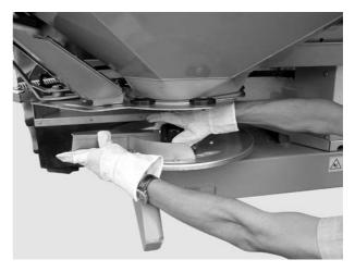
Figure 14: Screwing on the cap nuts
