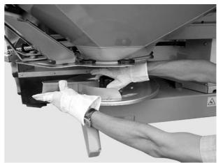
Figure 6: Unscrew the cap nut
