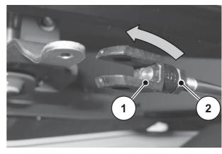
Figure 28: Disengaging the inner yoke
