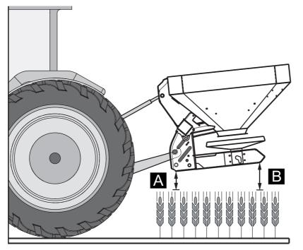
Figure 8.11: Mounting position and height during late fertilisation
