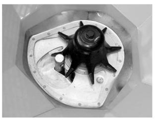
Take a lower link pin d = 28 mm and insert it centrally into the metering opening.
