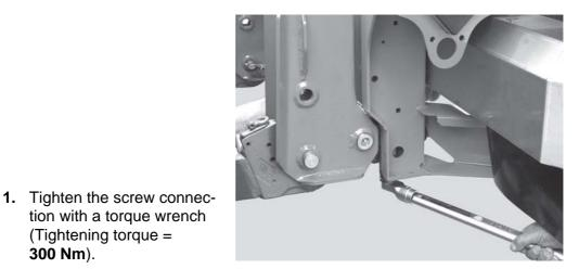
Figure 20: Fastening the weighing cell (on the left side of the direction of travel)
