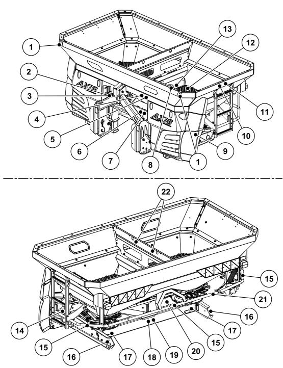
Figure 3.2: Position of protective devices, warning and instruction notices, and reflectors
