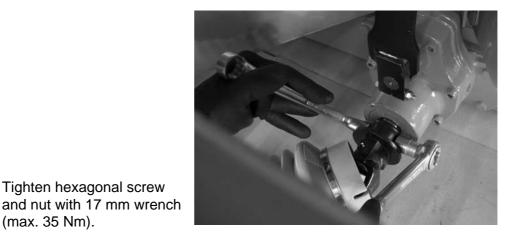
Figure 4: Tighten drive shaft
