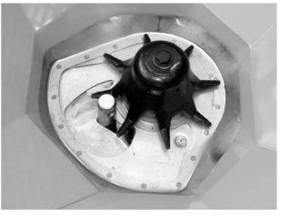
Figure 25: Lower link pin in metering opening
