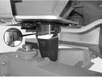
Figure 12: Attaching the calibration test chute
