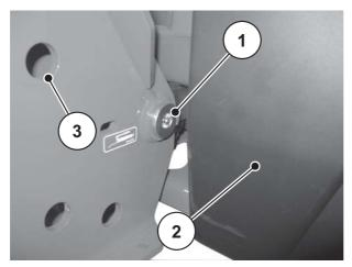
Figure 17: Lubrication point of weighing spreader
