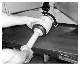
Figure 6: Put the universal drive shaft guard back on
