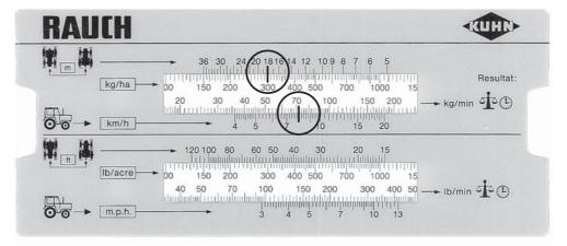
Figure 9: Scale for calculation of the nominal output volume per minute
