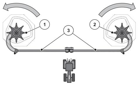
Figure 9.5: Checking the agitator drive
