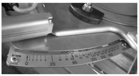
Figure 1: Scale for setting the spreading quantity
