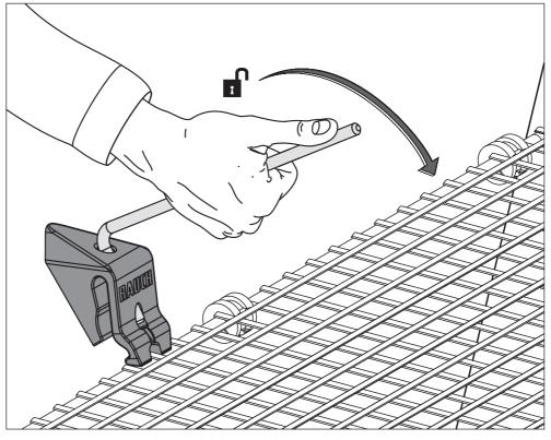
Figure 9.2: Opening the protective grid lock
