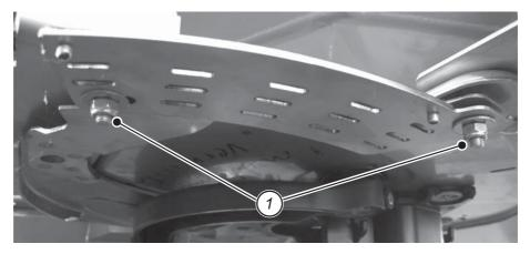
Figure 21: Scale fixing screws
