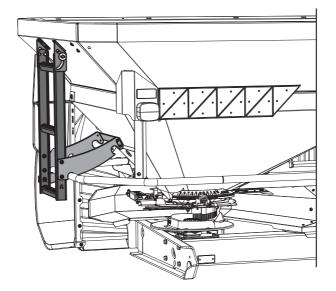
Figure 16: Folding in the steps in closed position
