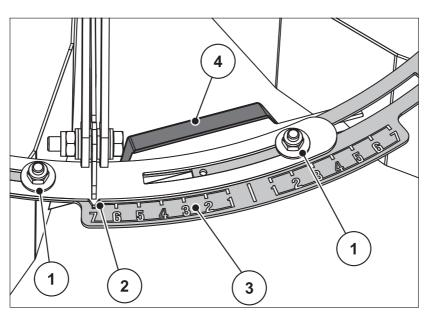
Figure 8.21: Setting the border spreading unit
