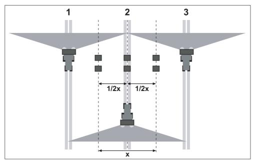
Figure 8.27: Layout for three passes
