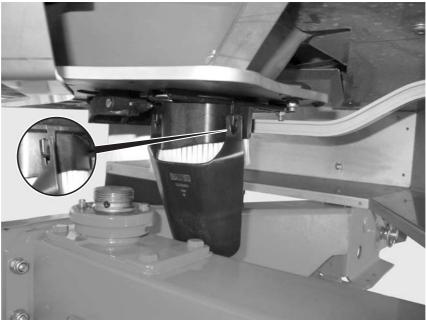
Figure 12: Attaching the calibration test chute
