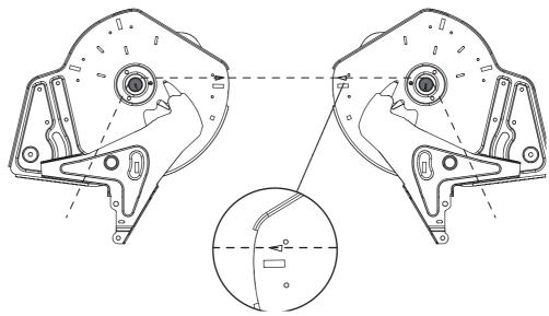
Figure 27: Checking the drop point
