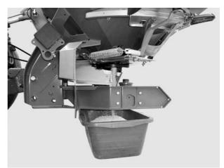
**5.** Position a collection vessel under the left output.
