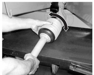
Figure 8.4: Put the universal drive shaft guard back on
