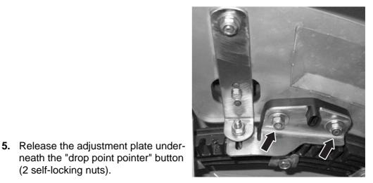
Figure 28: Loosen the drop point adjustment plate
