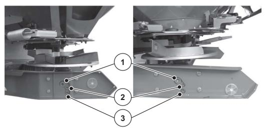
Figure 9.10: Gear oil filling and draining points; left: AXIS 20.1, AXIS 30.1, right AXIS 50.1
