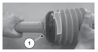
Loosen the universal drive shaft Figure 1: guard
