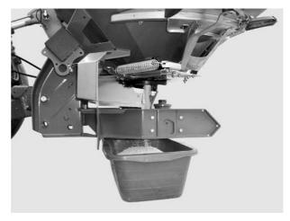
**3.** Position a collection vessel under the left output.
