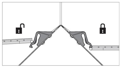
Figure 9.1: Protective grid lock open/closed
