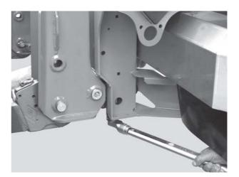
Figure 23: Fastening the weighing cell (on the left side of the direction of travel)
