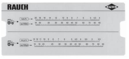
Figure 15: Scale for calculating the exact forward speed
