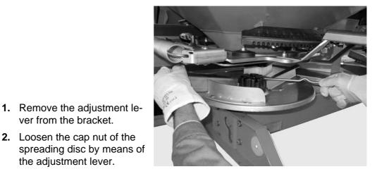
Figure 5: Loosen cap nut
