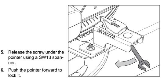
Figure 32: Setting the pointer manually
