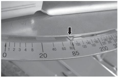
Figure 22: Metering slide pointer on position 85
