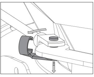
Figure 44: Removing the pin
