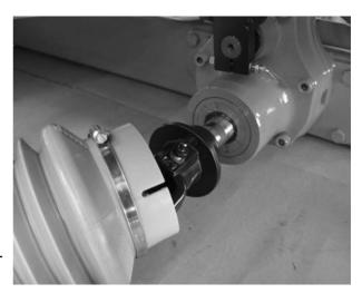
Figure 3: Push the universal drive shaft onto the transmission spigot
