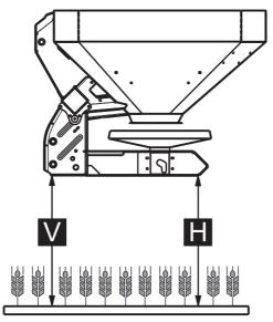
**Figure 8.9:** Maximum admissible mounting height V and H during normal and late fertilisation
