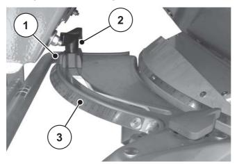
Figure 3: Adjustment scale for the spreading volume
