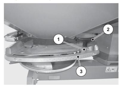
Figure 10: Adjustment scale for the spreading volume
