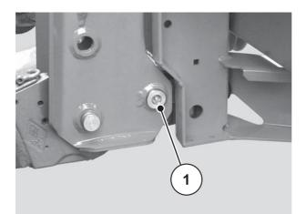
Figure 19: Lubrication point of weighing spreader
