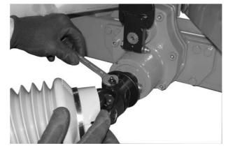
Figure 5: Tighten lubricating nipples
