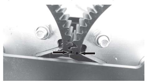
Figure 26: Underside of the toothed elements, markings must coincide: Markings must coincide
