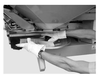
Figure 5: Unscrew the cap nut
