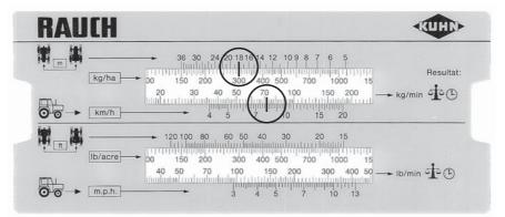
Figure 8: Scale for calculating the exact forward speed
