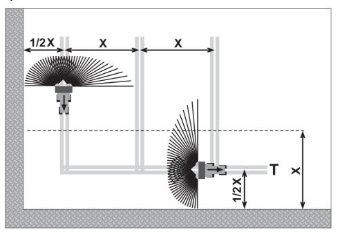
Figure 8.19: Environmentally optimised boundary spreading
