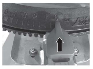
Bild 39: Set the drop point to position 0.
