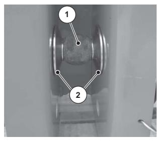
Figure 8.7: Position of the distance washers when installing the machine (AXIS 50.1, category III)
