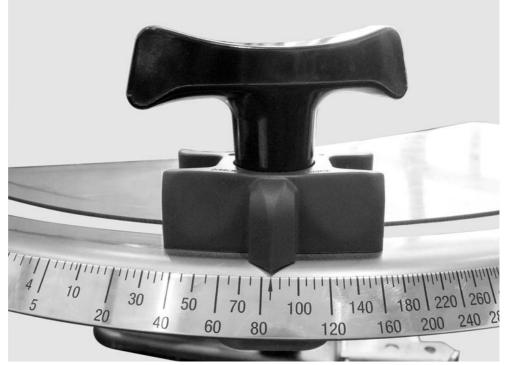
Figure 23: Adjustment scale of metering slide
