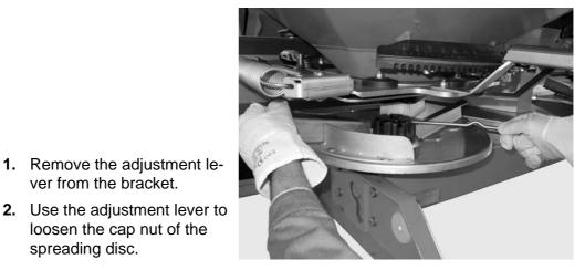
Figure 12: Loosen cap nut
