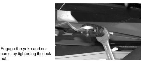
Figure 29: Engaging the inner yoke
