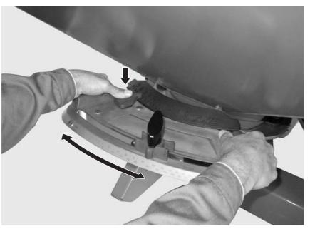
Figure 14: Adjustment centre for drop point
