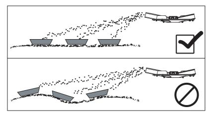
Figure 8.25: Layout of the catch trays
