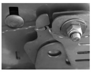
Figure 35: Attaching the string to the adjustment centre
