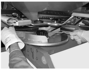
Figure 11: Loosen cap nut
