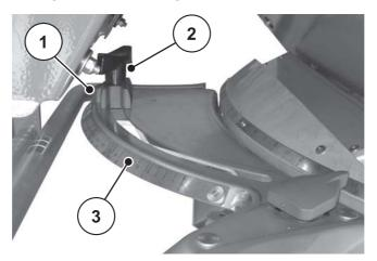
Figure 2: Adjustment scale for the spreading quantity
