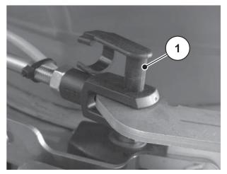
Figure 40: Engaging the outer yoke.
