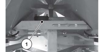
Figure 17: Calibration test chute
