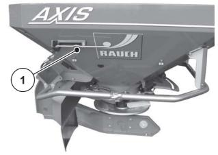
[1] Adjustment lever (hopper, left side according to direction of travel)
