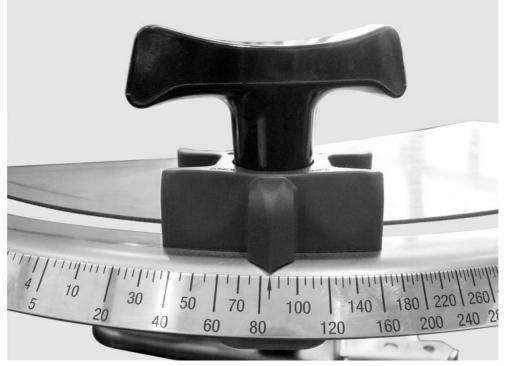
Figure 23: Adjustment scale of metering slide
