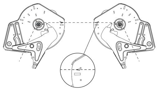
Figure 24: Checking the drop point
