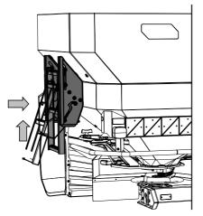
Figure 16: Folding in the steps in closed position
