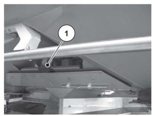
[1] Position of the calibration test chute
