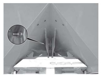
Figure 21: Fastening the tie rod (in the rear of the direction of travel underneath the intermediate roof)
