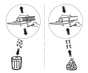
Figure 9.9: Use new self-locking nuts.
