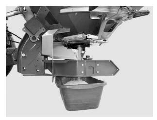
**5.** Position a collection vessel under the left output.
