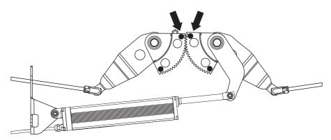
Figure 25: Position of the markings on the toothed segments
