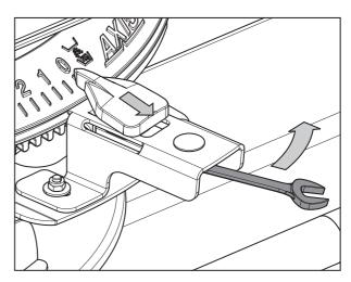
Figure 41: Pushing the pointer back again
