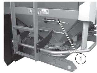
[1] Adjustment lever (hopper, left side according to direction of travel)
