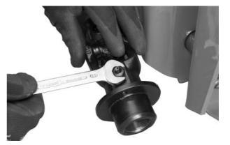
Remove lubricating nipples Figure 2:
