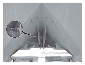
Figure 24: Fastening the tie rod (in the rear of the direction of travel underneath the intermediate roof)
