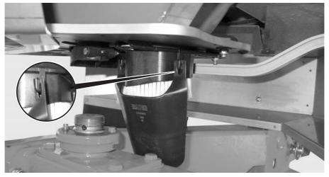
Figure 19: Attaching the calibration test chute
