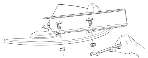
Figure 9.8: Remove the vane screws
