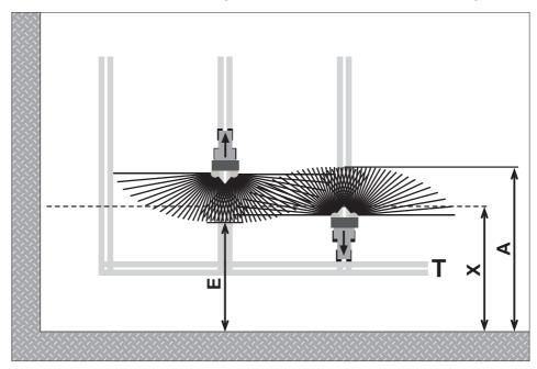
• Move the border spreading unit TELIMAT out of the spreading area.
