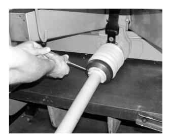
Figure 7: Secure universal drive shaft guard
