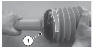
Figure 8.1: Loosen the universal drive shaft guard
