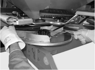
Figure 18: Loosen cap nut
