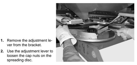
Figure 4: Loosen cap nut
