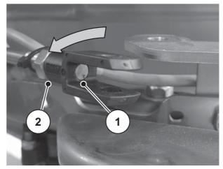
Figure 30: Disengaging the outer yoke
