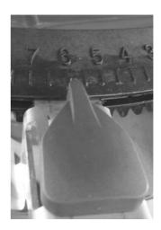
4. Set the drop point to position 6 by turning the adjustment centre on both sides.
