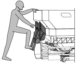
Figure 17: Climbing onto the machine without hopper cover
