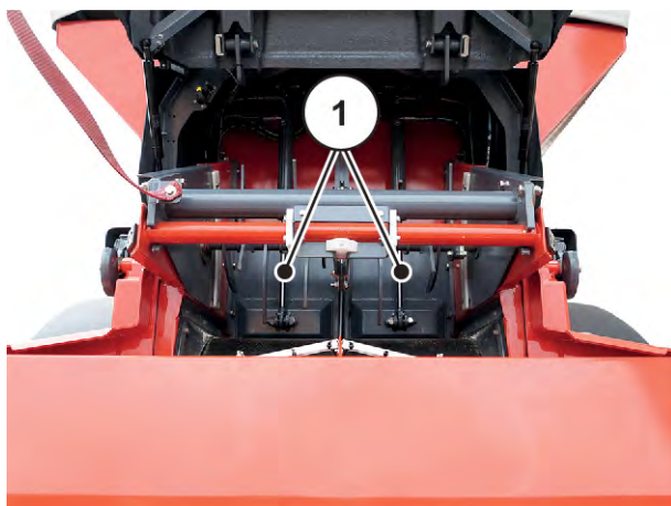
Fig. 49: Pre-metering slide in closed position
