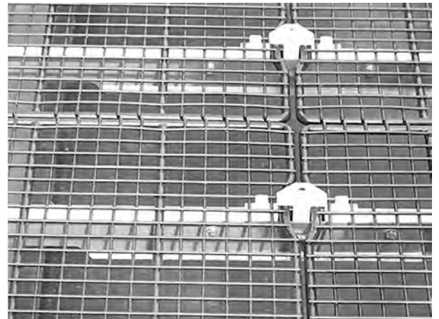
Fig. 41: Feeder mesh in hopper
