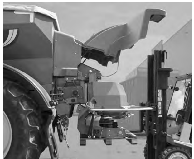
Fig. 43: Positioning the forklift truck
