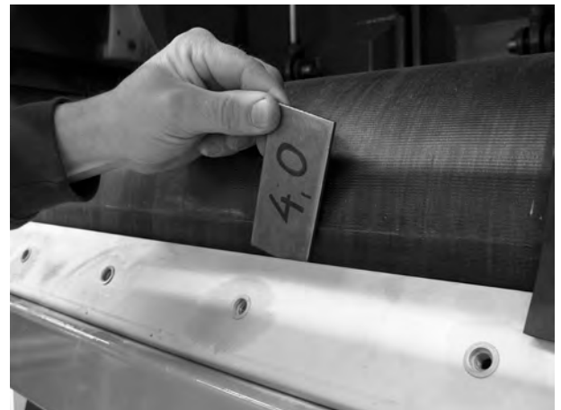
Fig. 122: Checking the clearance
