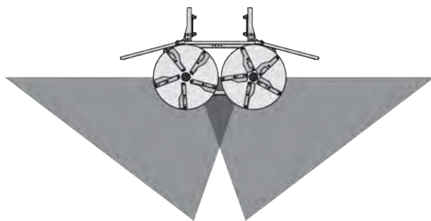
Fig. 72: Normal spreading pattern, drop point in the neutral position
