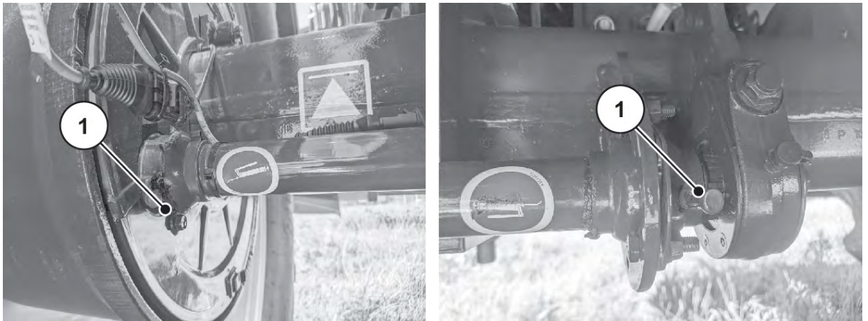
Fig. 92: Rigid axle brake camshaft bearing
